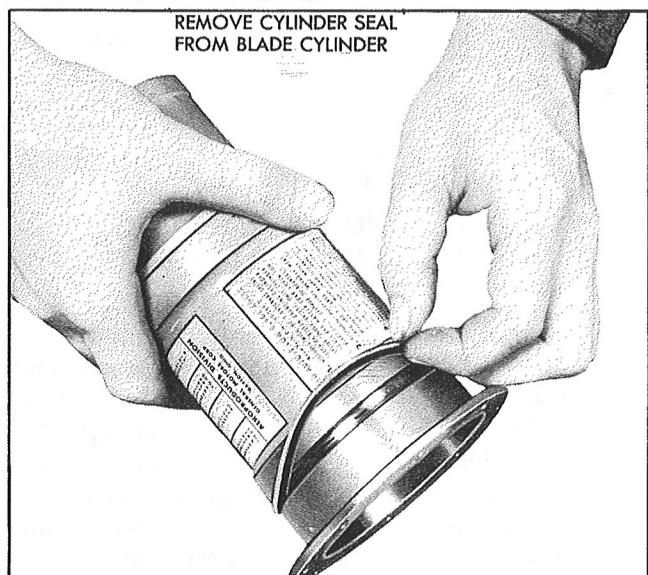
Figure 110—Removal of the Blade Cylinder Seal
