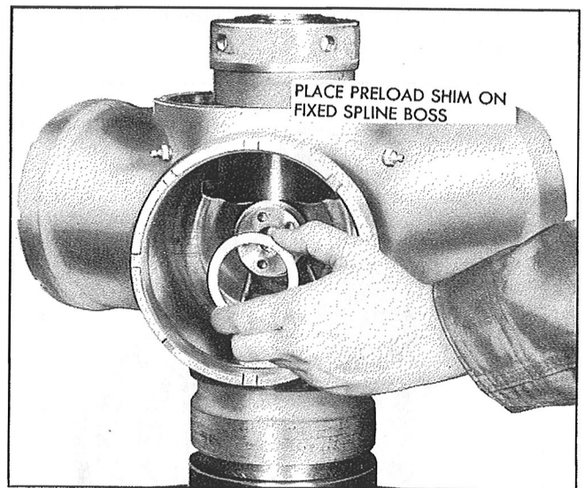
Figure 113—Installation of the Pre-load Shim
